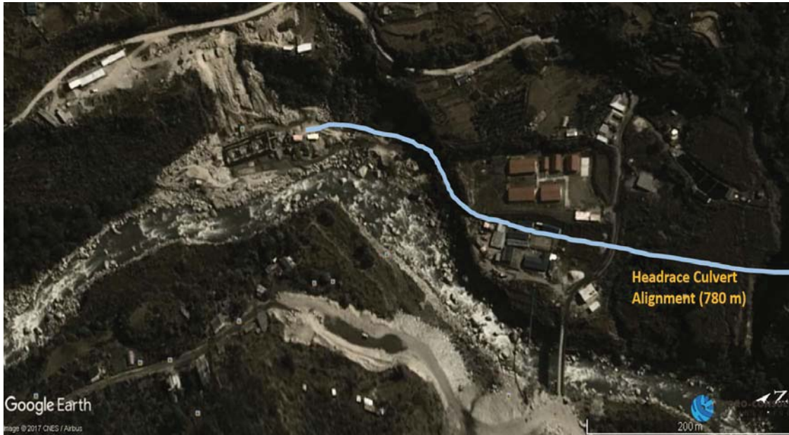
MISTRI KHOLA-2 HEP HEADRACE CULVERT ALIGNMENT
